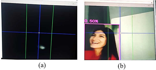
Fig. 9. Two shots of the real-time object detection test based on different light degrees. (a) The failure of object detection in darkness. (b) A person is detected in the lightness.
