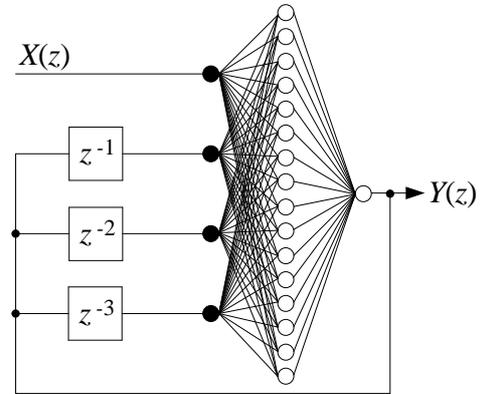
Fig. 5. Multilayer neural network NEWFF structure.
