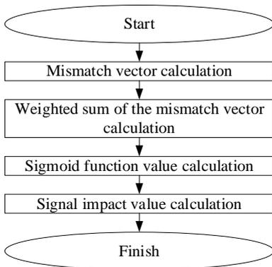
Fig. 4. Block diagram of the algorithm of the adaptation module with signal adaptation.
