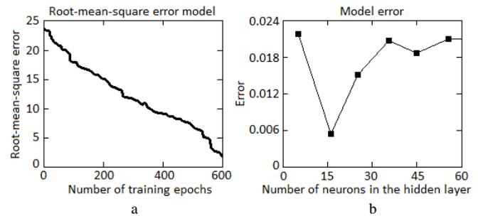
Fig. 7. Results of training the neural network: a – characteristic of the accuracy of training the neural network; b – dependence of training error on the complexity of the neural network.
