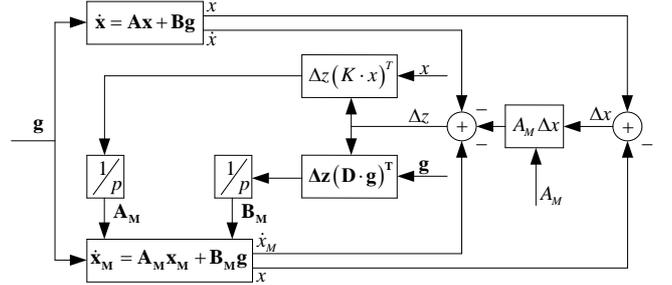
Fig. 1. Block diagram of real-time identification (developed by V. Bakhirev).
