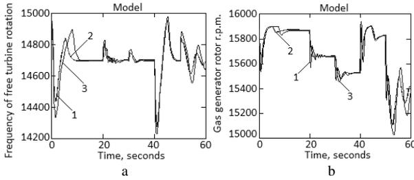
Fig. 8. Diagram of change: a – frequency of free turbine rotation; b – gas generator rotor r.p.m.
