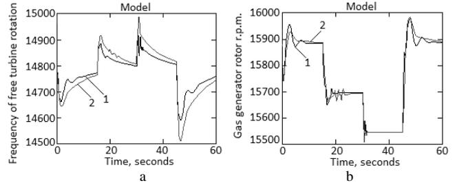
Fig. 10. Diagram of change: a – frequency of free turbine rotation; b – gas generator rotor r.p.m.
