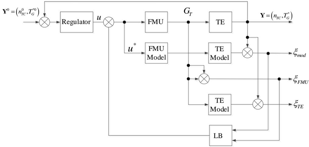
Fig. 2. Helicopters TE automatic control system [10].
