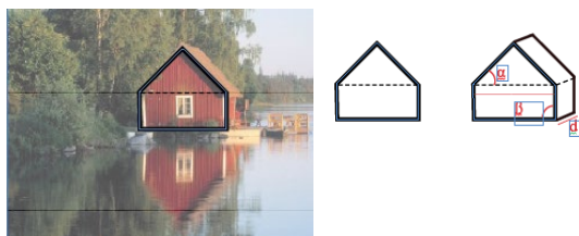
Figure 1: left) a typical Norwegian cabin outline (svenskoedegaard, 2020), and right) the extracted geometry showing different parameters.
