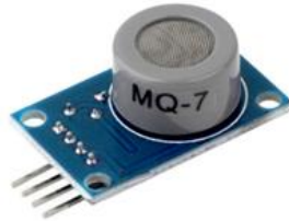
Figure 1 Carbon Monoxide MQ-7 Sensor [4-5]
