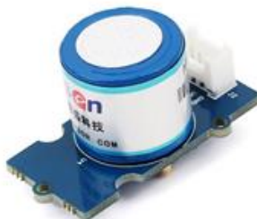
Figure 3 Oxygen ME2 - O2 Sensor [8-9]
