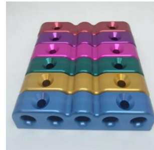
Fig. 4 Photographs of titanium products subjected to combined etching after electrochemical oxidation in a solution of tartaric acid. Final voltage on the cell from 30 to 120 V
