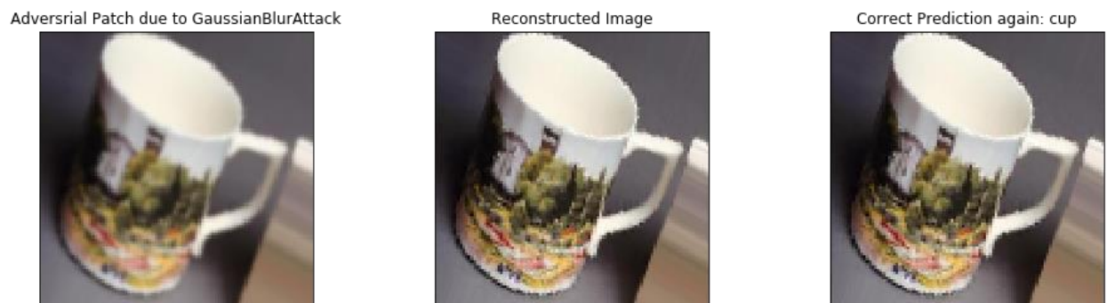
Fig20. (a) Adversarial image created due to Gaussian Blur Attack. (b) Reconstructed adversarial image by applying our proposed method. (c) Our model predicts correct label cup of reconstructed adversarial image again.
