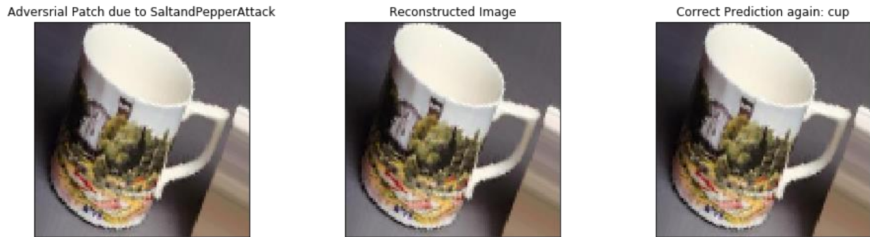
Fig24. (a) Adversarial image created due to Salt and Pepper Noise Attack. (b) Reconstructed adversarial image by applying our proposed method. (c) Our model predict correct label cup of reconstructed adversarial image again.
