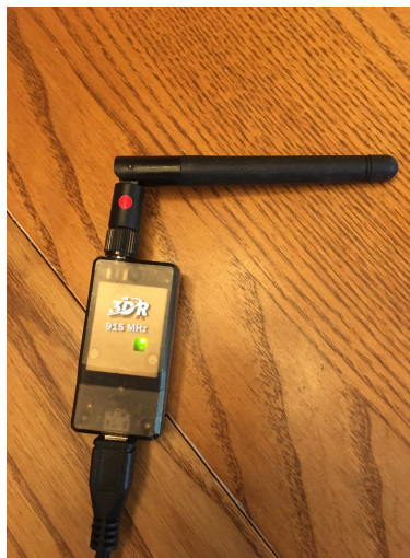
Figure 16: Blinking Green Light on Telemetry system proves it is operating correctly
