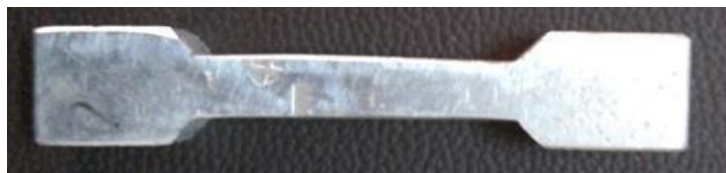
Figure 1 Developed nano-carbon doped aluminium oxide sample as per ASTM D 638-03 size.
