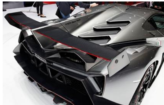
Fig. 2 Thermoplastic polymer matrix composite material used in the rear wing of the race car [9-10].
