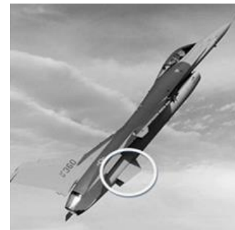
Fig. 9 The rear body wings of the F16 are made of Al matrix composites [22].
