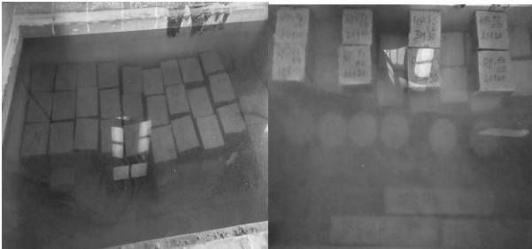
Fig 5:- Prepared specimens are curing
