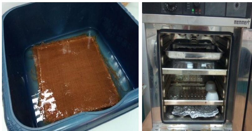
Fig. 2. Impregnation of jute fabrics in the 5% NaOH / 2 h solution with T^\circ = (30, 60, 90, 120, 160 and 200)^\circ\text{C}
