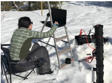
Figure 3.3: Data collection using an external computer in serial communication with the prototype.
