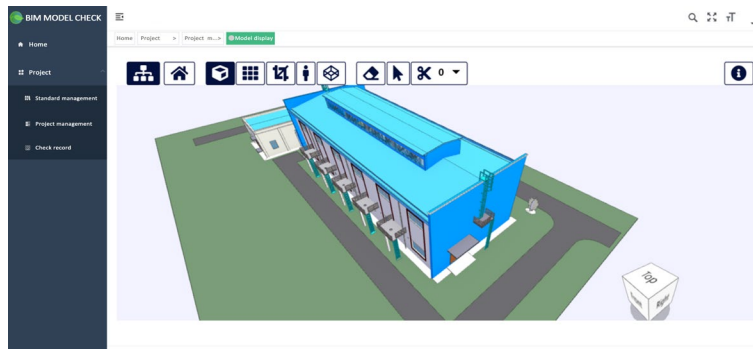
Figure 9: Compliance check platform for BIM models
