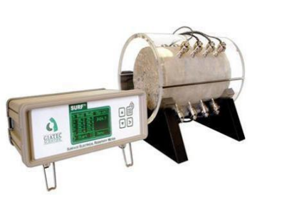
Figure 1: Wenner device for surface resistivity measurement
