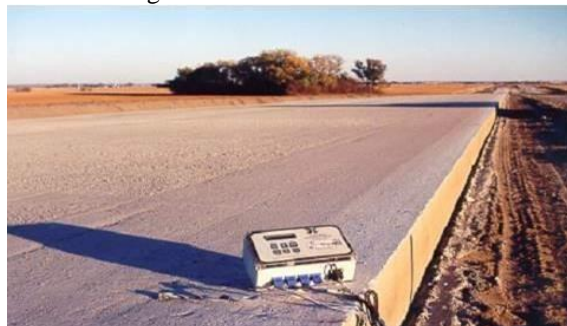
Figure 2: Maturity measurement of concrete (US DOT, 2000)
